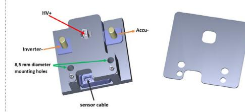
SENSOR ASSEMBLY WITH COVER AND CABLE LUGS:
