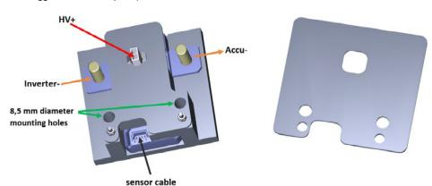
SENSOR ASSEMBLY WITH COVER AND CABLE LUGS:
