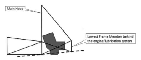
The engine lubrication system must be protected from surface contact in any situation while in operation on track, especially in case of a suspension failure. The skid plate itself can not be mounted to parts of the engine.
