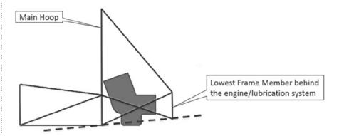
The engine lubrication system must be protected from surface contact in any situation while in operation on track, especially in case of a suspension failure. The skid plate itself can not be mounted to parts of the engine.
